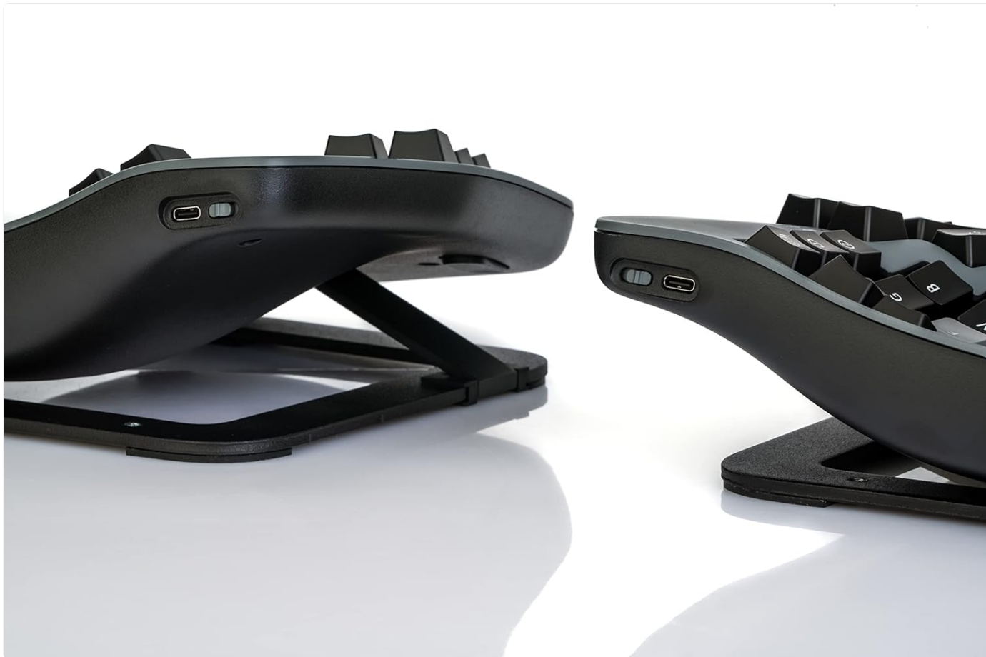
Figure 3.1: USB-C ports on the keyboard halves for charging and wired connection.
