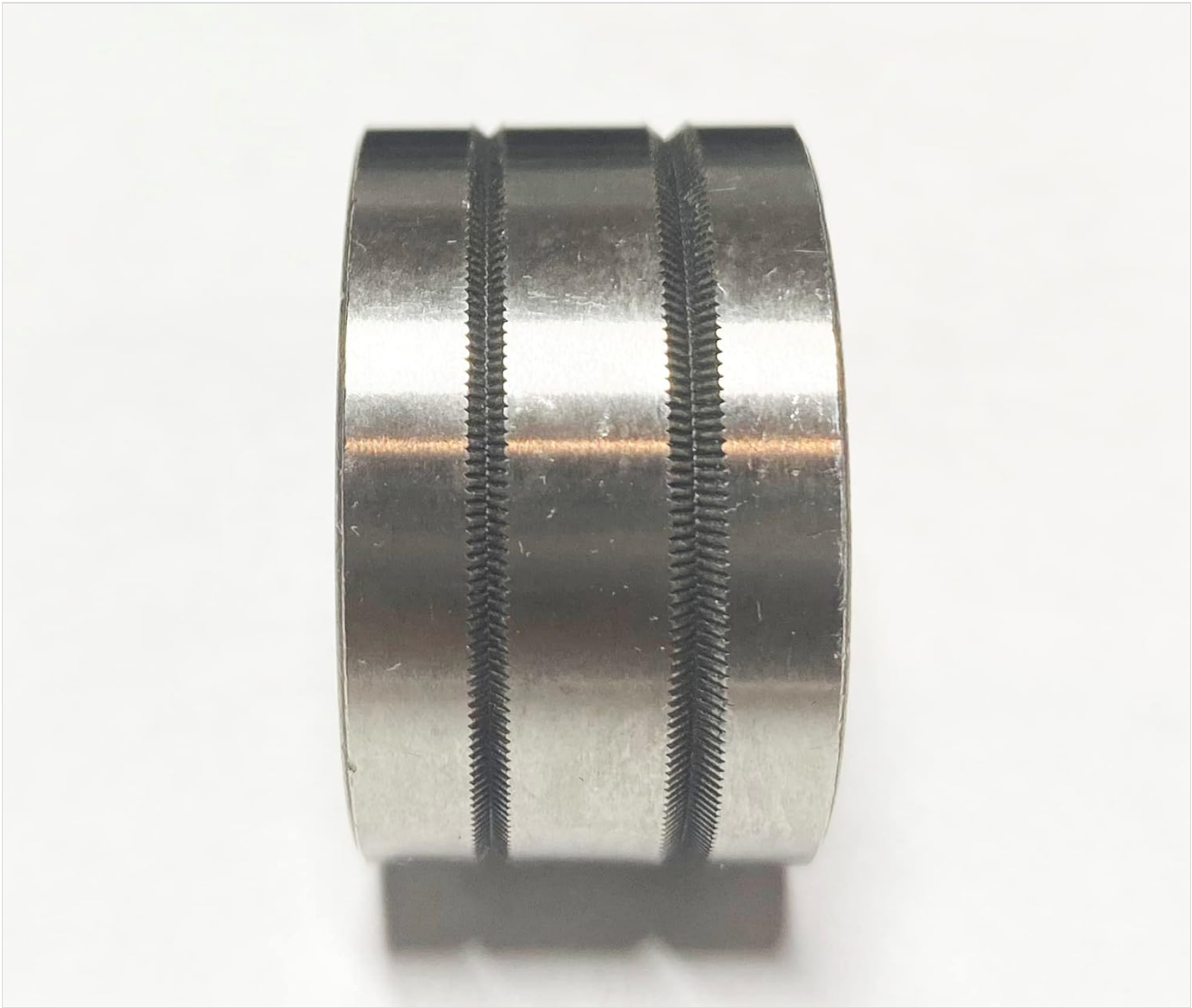
Figure 3.2: Side profile of the drive roll, illustrating the two distinct V-grooves for different wire diameters. The knurled edges provide traction for wire feeding.
