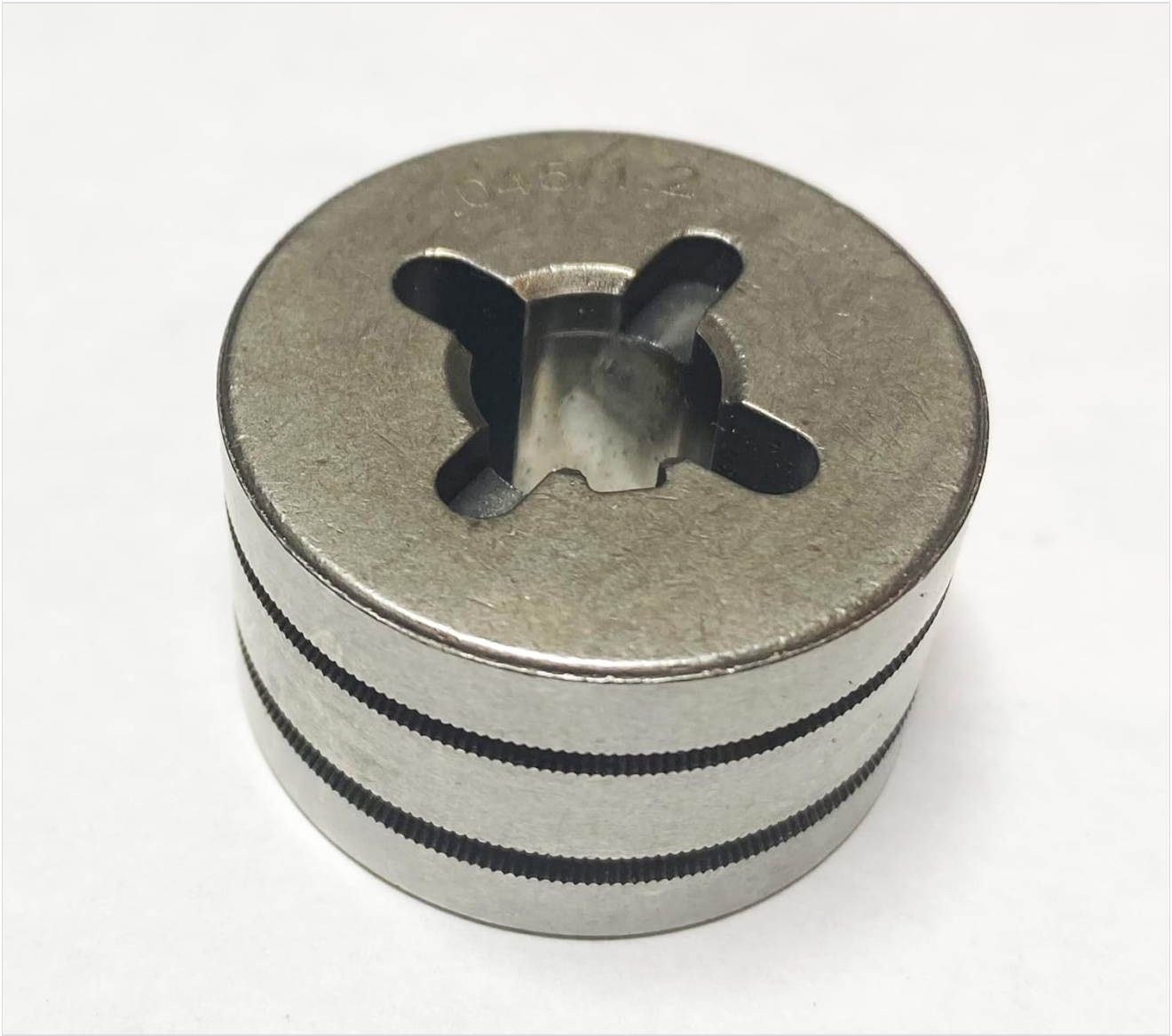
Figure 3.3: Rear view of the drive roll, showing the .045 (1.2) wire size marking. This side is used when feeding .045 inch wire.
