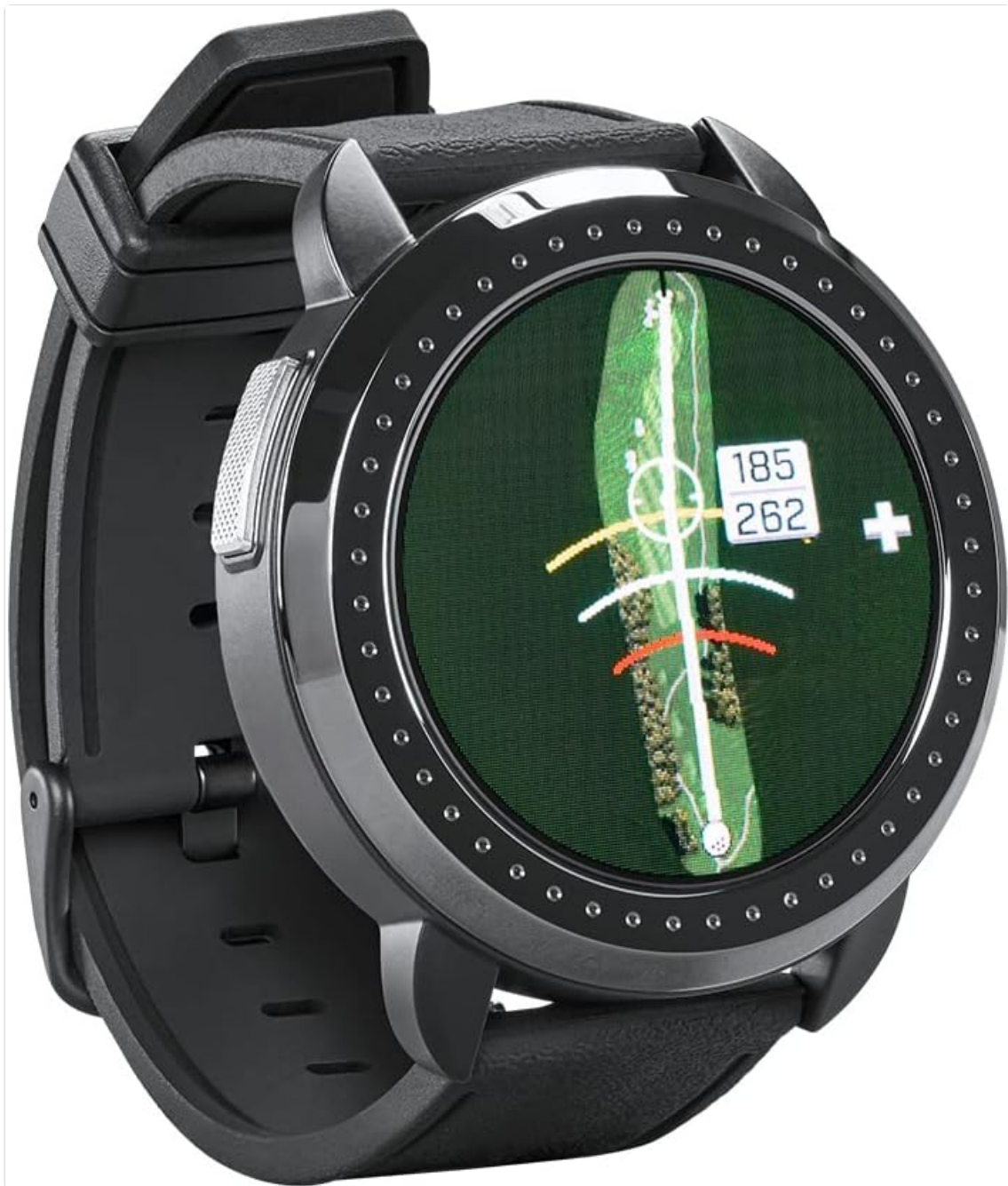
Figure 5: HoleView feature showing the hole layout and shot planning options.
