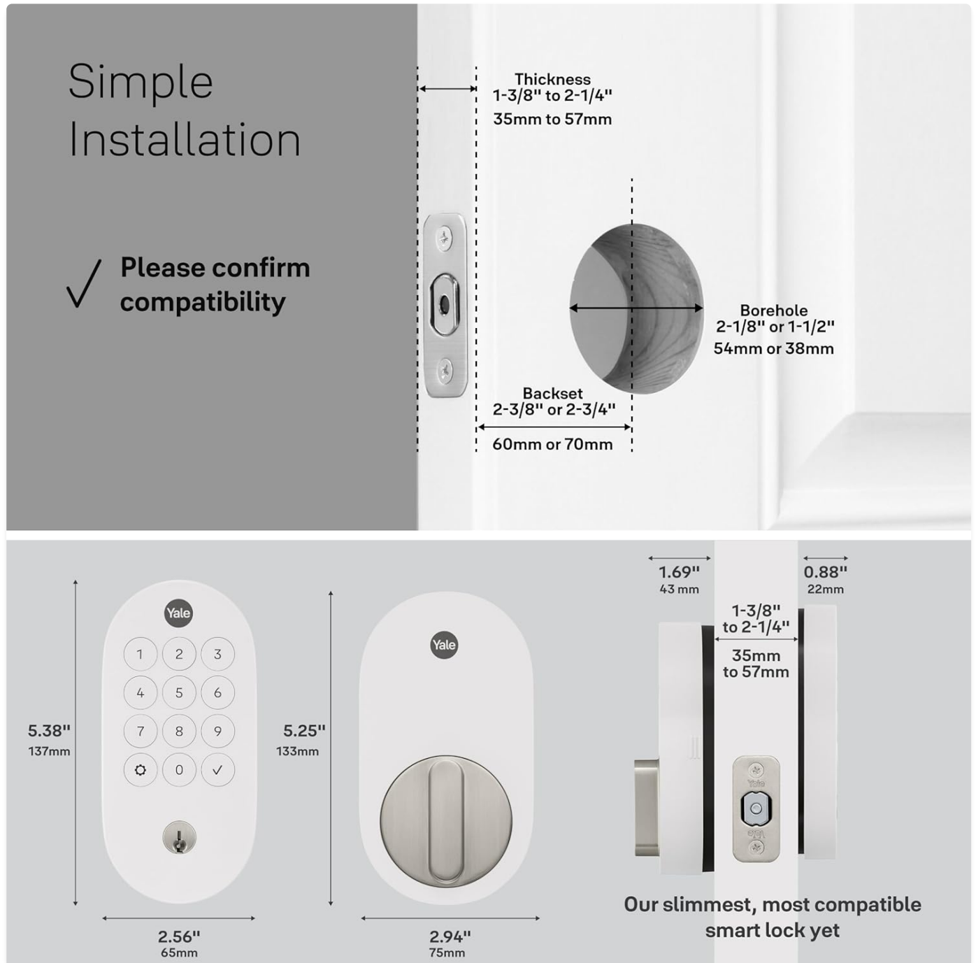
Image: A diagram illustrating the required door dimensions for Yale Smart Lock installation, including door thickness (1-3/8" to 2-1/4"), bore hole diameter (2-1/8" or 1-1/2"), and backset (2-3/8" or 2-3/4").
