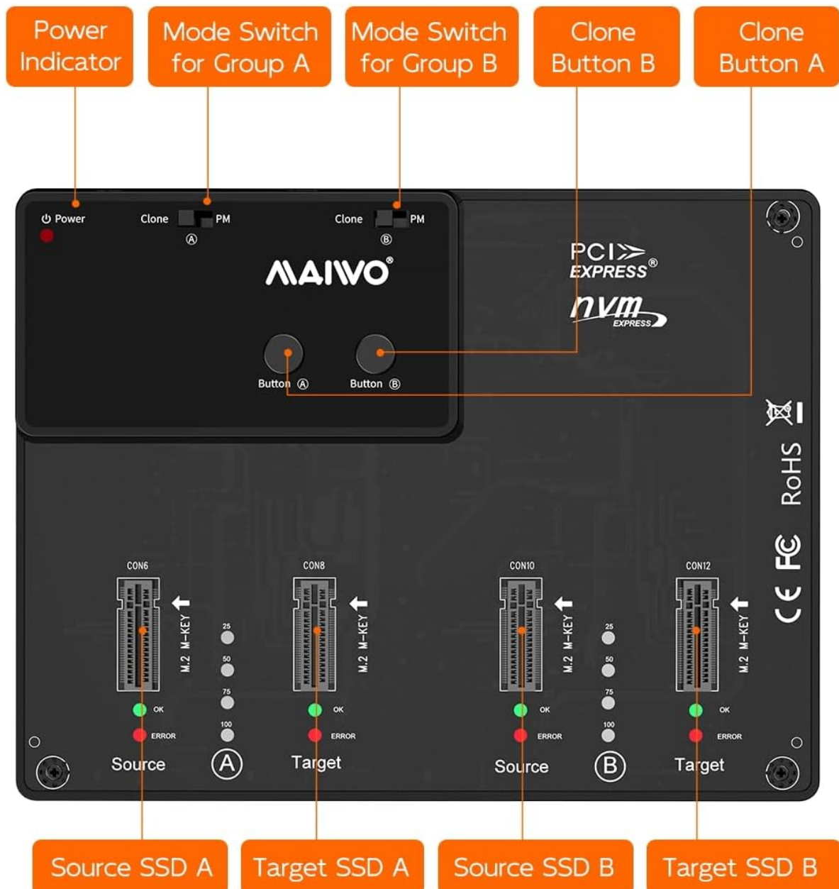
Image 3.1: Labeled diagram of the MAIWO M.2 NVMe SSD 4-Bay Docking Station.
