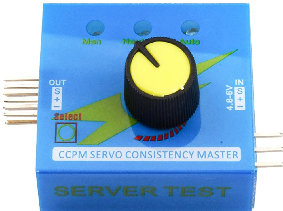
Image 5.1: Visual representation of the three modes: Manual Mode, Neutral Mode, and Automatic "Window Wiper" Mode, as indicated by the LEDs on the tester.
