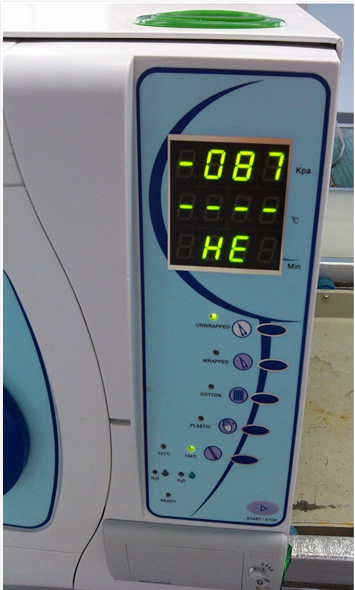
Figure 5.1: The control panel, displaying temperature, pressure, and time, along with program selection buttons.
