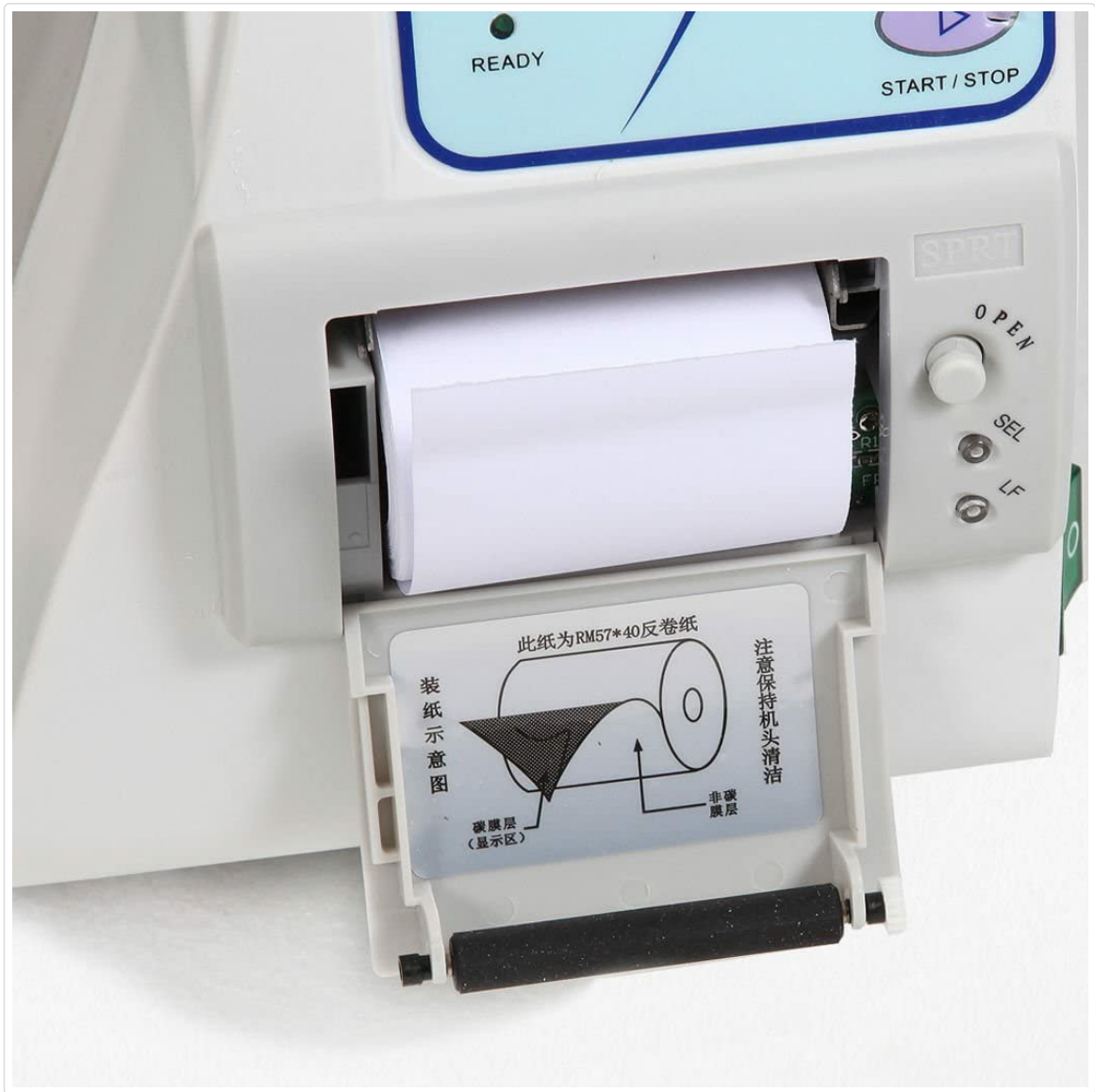
Figure 4.3: The integrated printer compartment, showing the paper roll and a diagram for correct paper loading.
