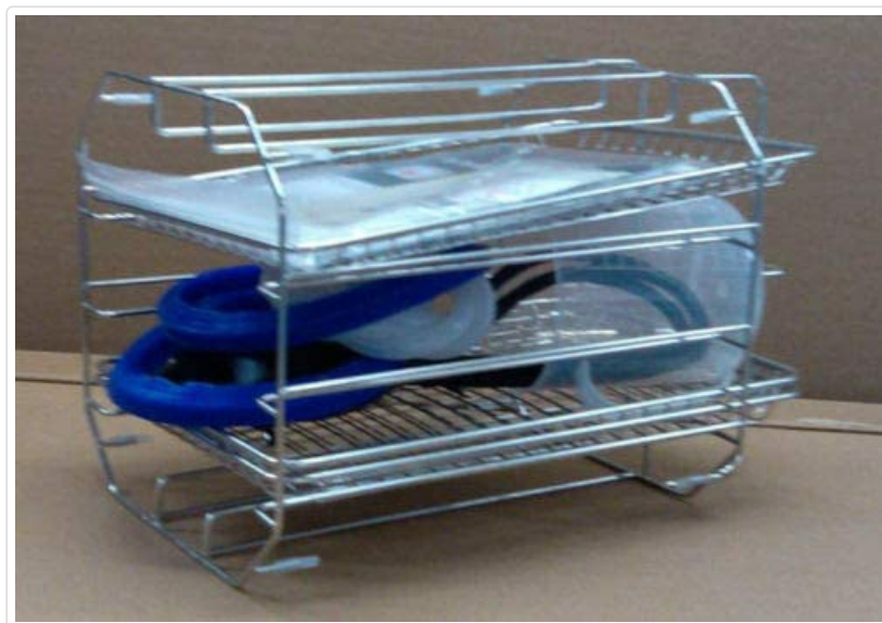
Figure 3.3: The metal instrument rack designed to hold items within the autoclave chamber.
