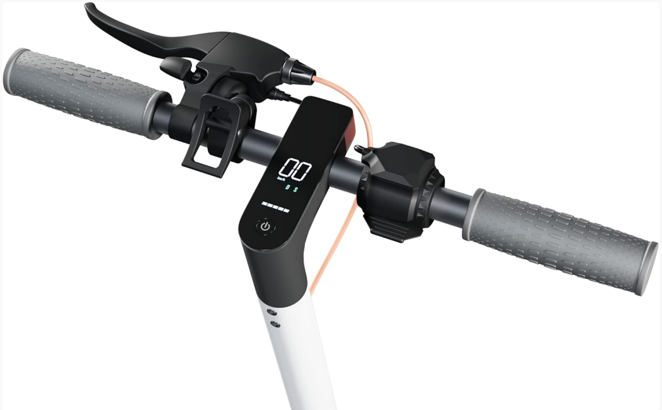
Figure 3.3: Close-up view of the handlebar, showing the LCD display, throttle, and brake lever.
