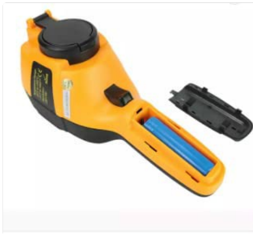
Figure 3.1: Opening the battery compartment and inserting the rechargeable battery.
