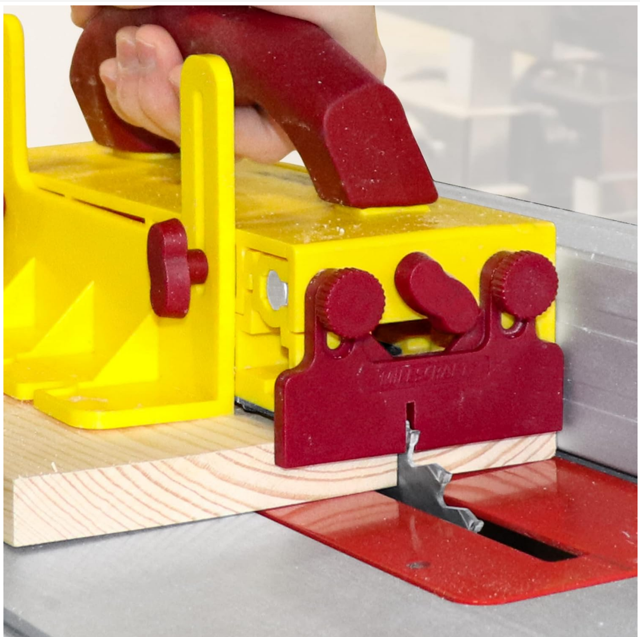
Figure 7: Proper use of the GrabberPRO on a table saw. This image demonstrates how the GrabberPRO is positioned over the
