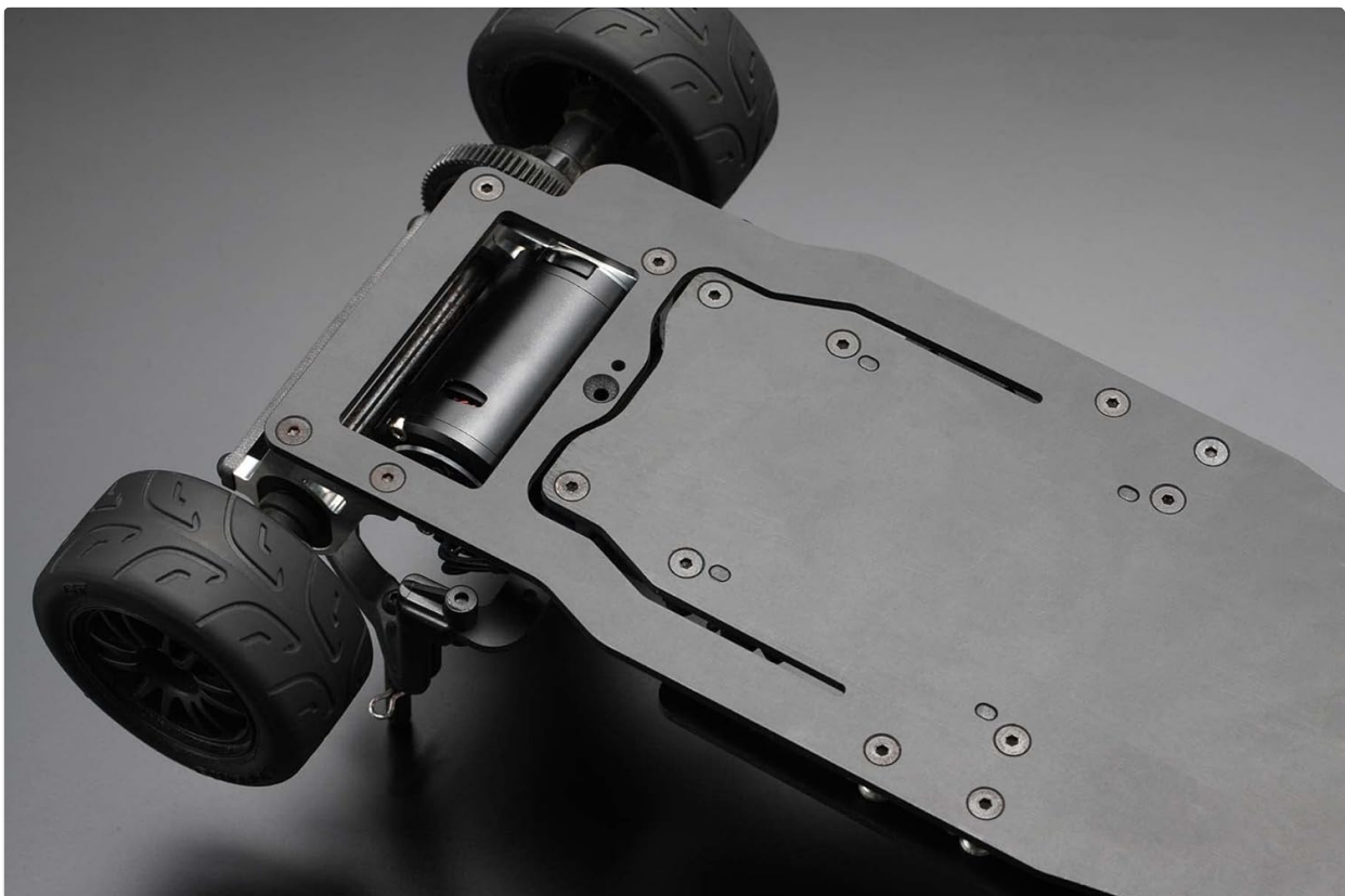
Figure 1.2: Bottom view of the GT1-01 chassis, illustrating the flat design and screw placements for various components.
