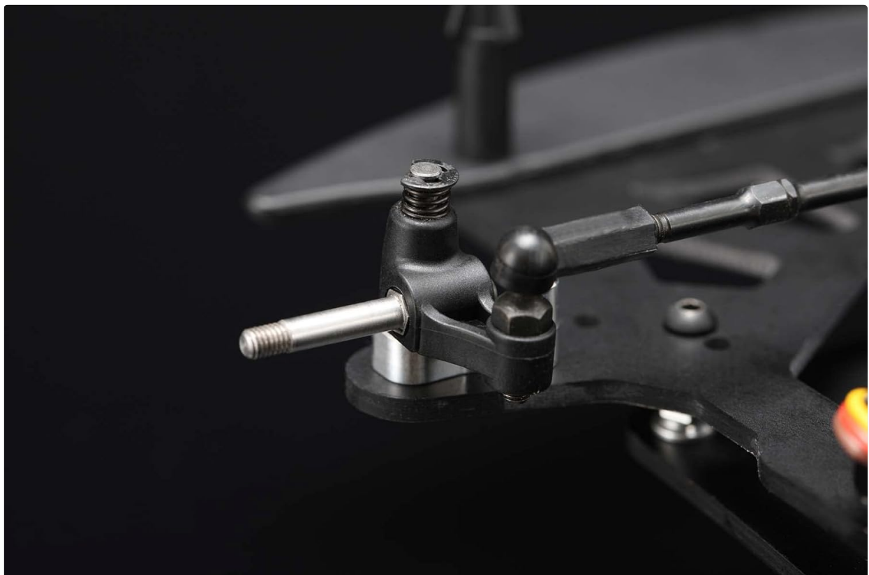
Figure 1.4: Detailed view of the front steering knuckle assembly, showing the pivot and linkage connection.
