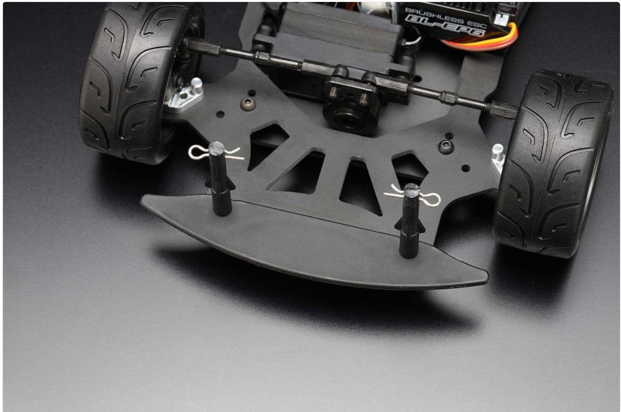
Figure 1.3: Detail of the front bumper and body post mounting points, secured with pins.
