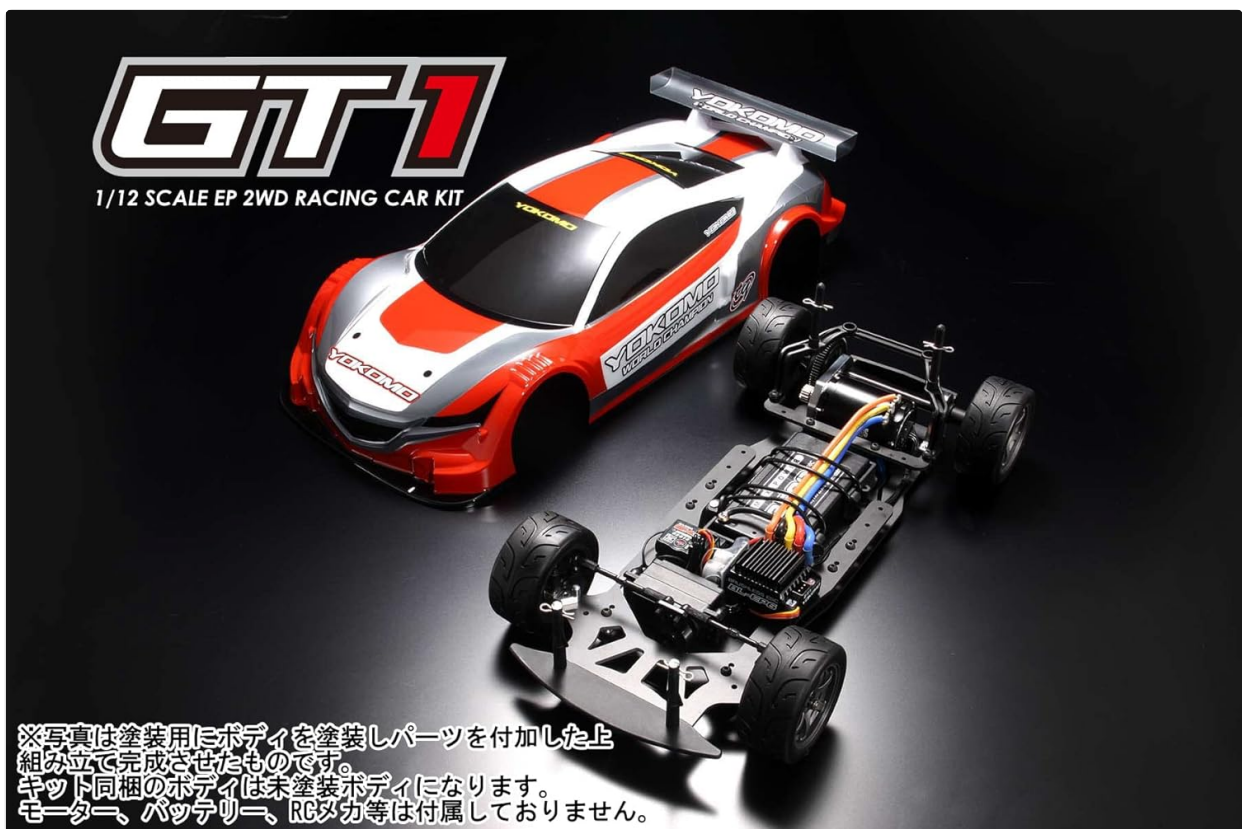
Figure 1.1: Overview of the Yokomo GT1-01 kit, showing the unpainted body and the assembled chassis with electronics installed (electronics not included in kit).
