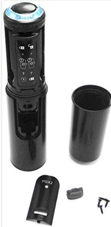
Figure 3.1: The HUMARH Handheld Body Shell assembled, ready for use with the Shure PGX2 Wireless Microphone's internal components.
