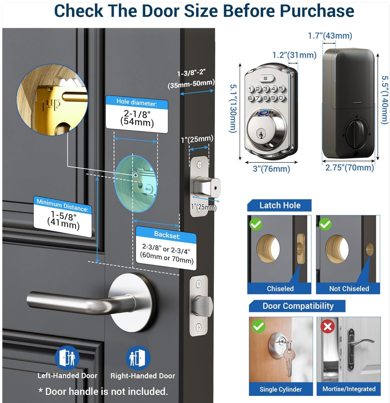
Figure 2.1: Door Size Compatibility Diagram. Ensure your door meets these specifications for proper installation.
