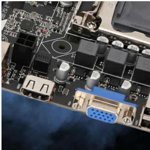
Figure 3.5: Close-up of the VGA and HDMI ports for connecting display devices.
