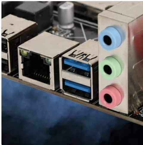
Figure 3.4: Detailed view of the rear I/O panel, including USB ports, Ethernet port, and audio jacks.
