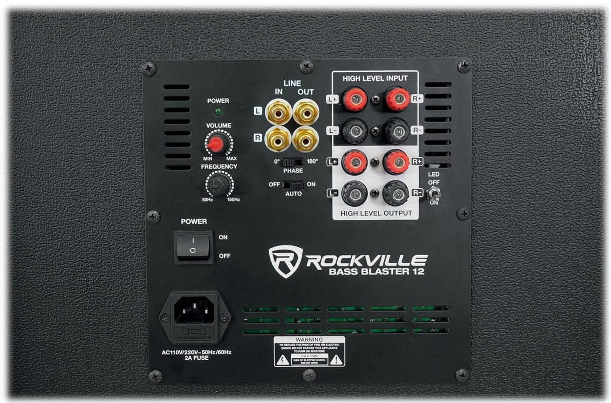
Figure 4: A detailed view of the rear panel controls on the Rockville BASS Blaster 12, including knobs for volume and frequency, and switches for phase and auto power.
