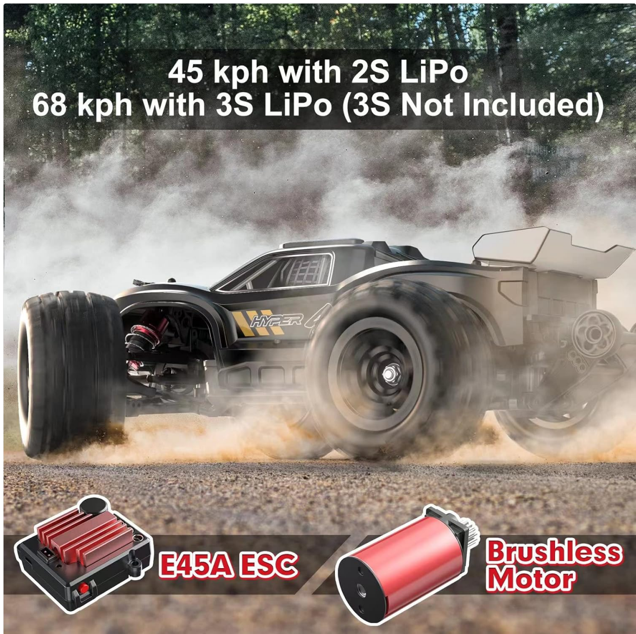
Figure 7: The powerful Hobby 2845 4200KV brushless motor and E45A ESC.
