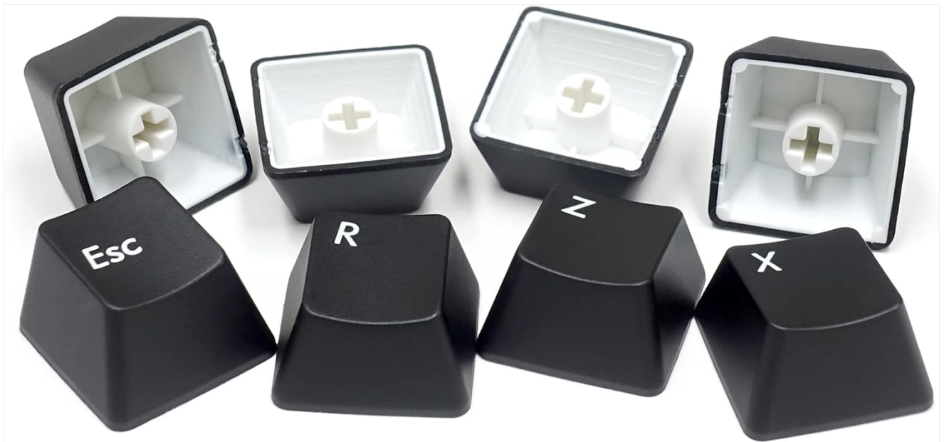
Image: Several PBT double shot keycaps removed from the keyboard, showing their construction and the Cherry MX compatible stems.
