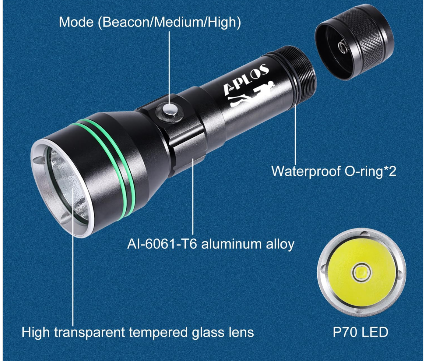
Image 4.1: Diagram illustrating the key components of the APLOS AP50 dive light, including the P70 LED, high transparent tempered glass lens, AL-6061-T6 aluminum alloy body, mode switch button, and waterproof O-rings.
