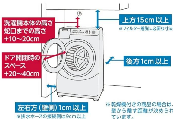
Figure 2.1: Installation Space Requirements and Dimensions
