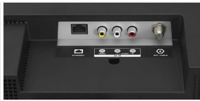
Image 4.2: Close-up of the bottom rear ports on the Insignia TV. This section shows the Ethernet port, AV IN (Video, L-Audio, R-Audio), and ANT/CABLE input.
