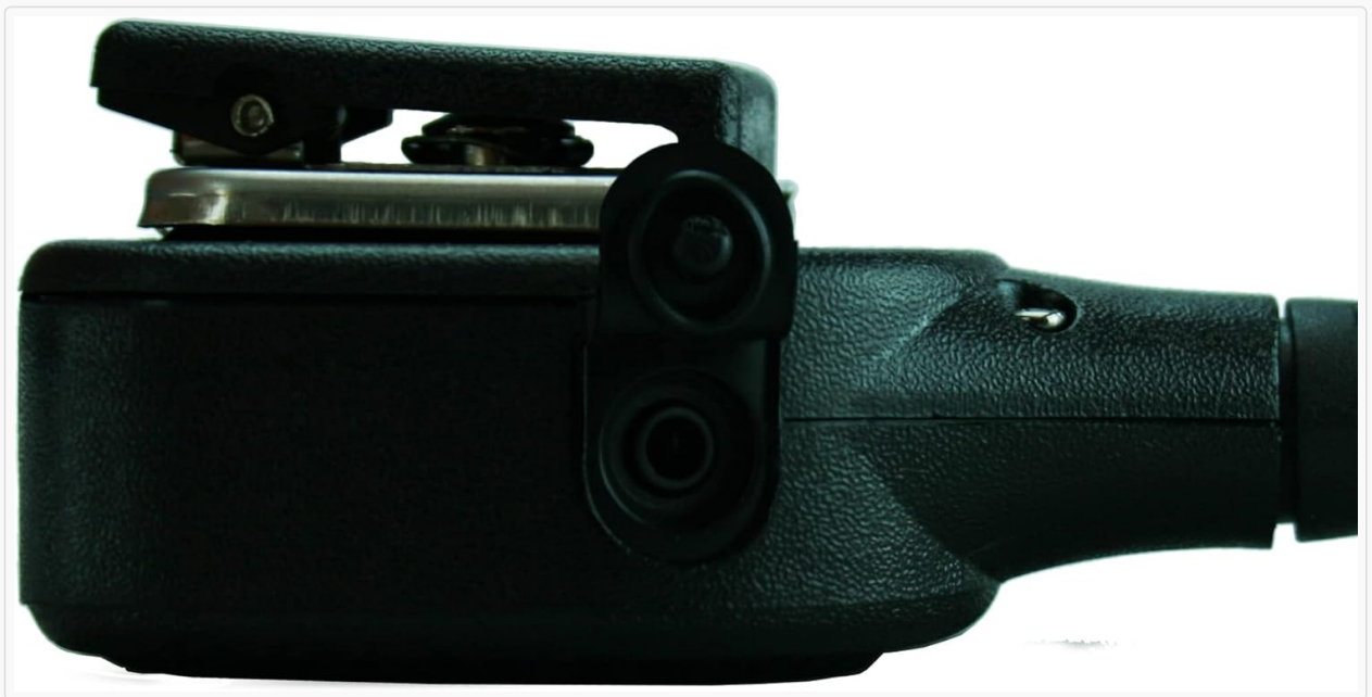
Figure 3.3: Side view of the microphone, indicating the 3.5mm audio jack for earpiece connection.
