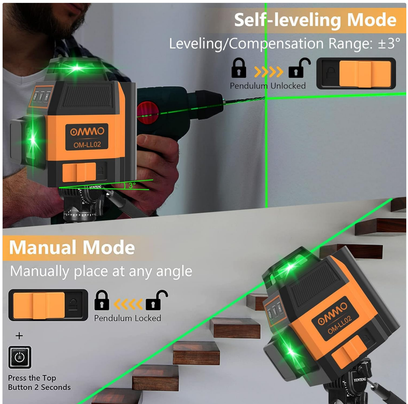
Image: Illustrates the side switch for pendulum lock/unlock, and how to activate self-leveling mode (unlocked) and manual/tilt mode (locked, then press top button).
