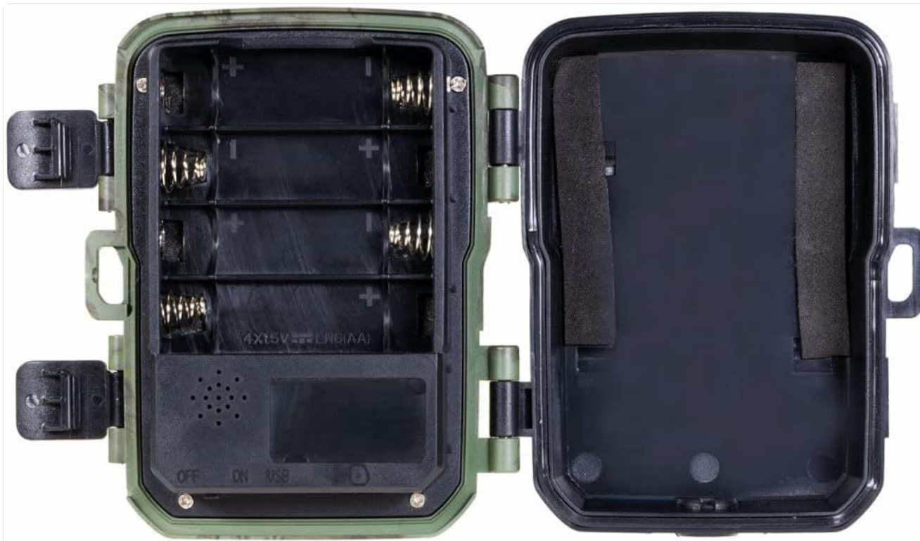
Image 4.1: Battery compartment and Micro SD card slot inside the camera.
