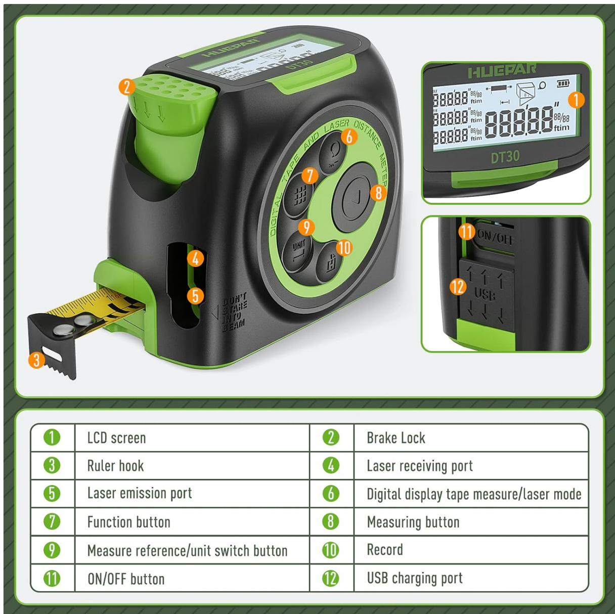
Image 3.1: Labeled components of the Huepar DT30.
