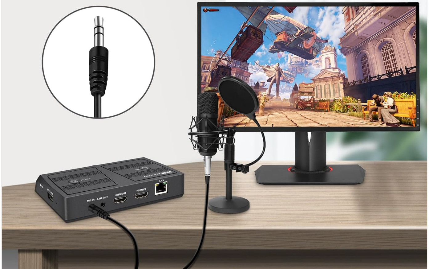
Image: Setup demonstrating how to record live commentary using a 3.5mm TRS microphone or headset connected to the capture board.
