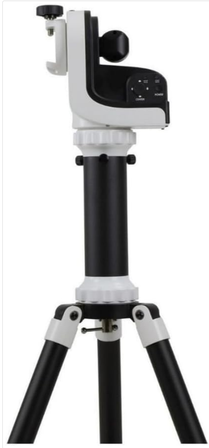
Figure 3: Close-up view of the SolarQuest mount's control panel, showing the 'POWER' button and the 8-way joystick for fine-tuning the telescope's position.
