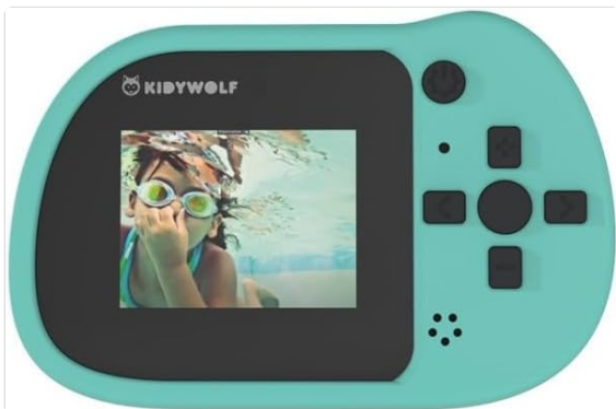
Image 1.2: Back View. This image shows the rear of the KIDYCAME, featuring the 2-inch LCD screen where captured images and videos are displayed. To the right of the screen are the control buttons for navigation and operation.
