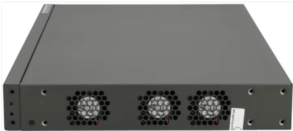
Figure 2.5: Side view of the Fiberhome S4820-X Series Switch, showing cooling fan vents for heat dissipation.
