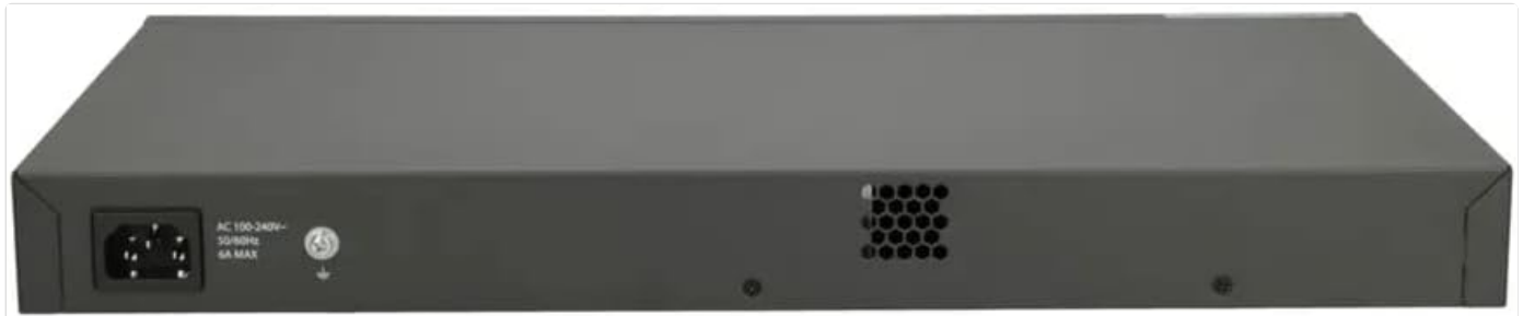
Figure 2.4: Rear panel of the Fiberhome S4820-X Series Switch, featuring the AC power input and grounding point.
