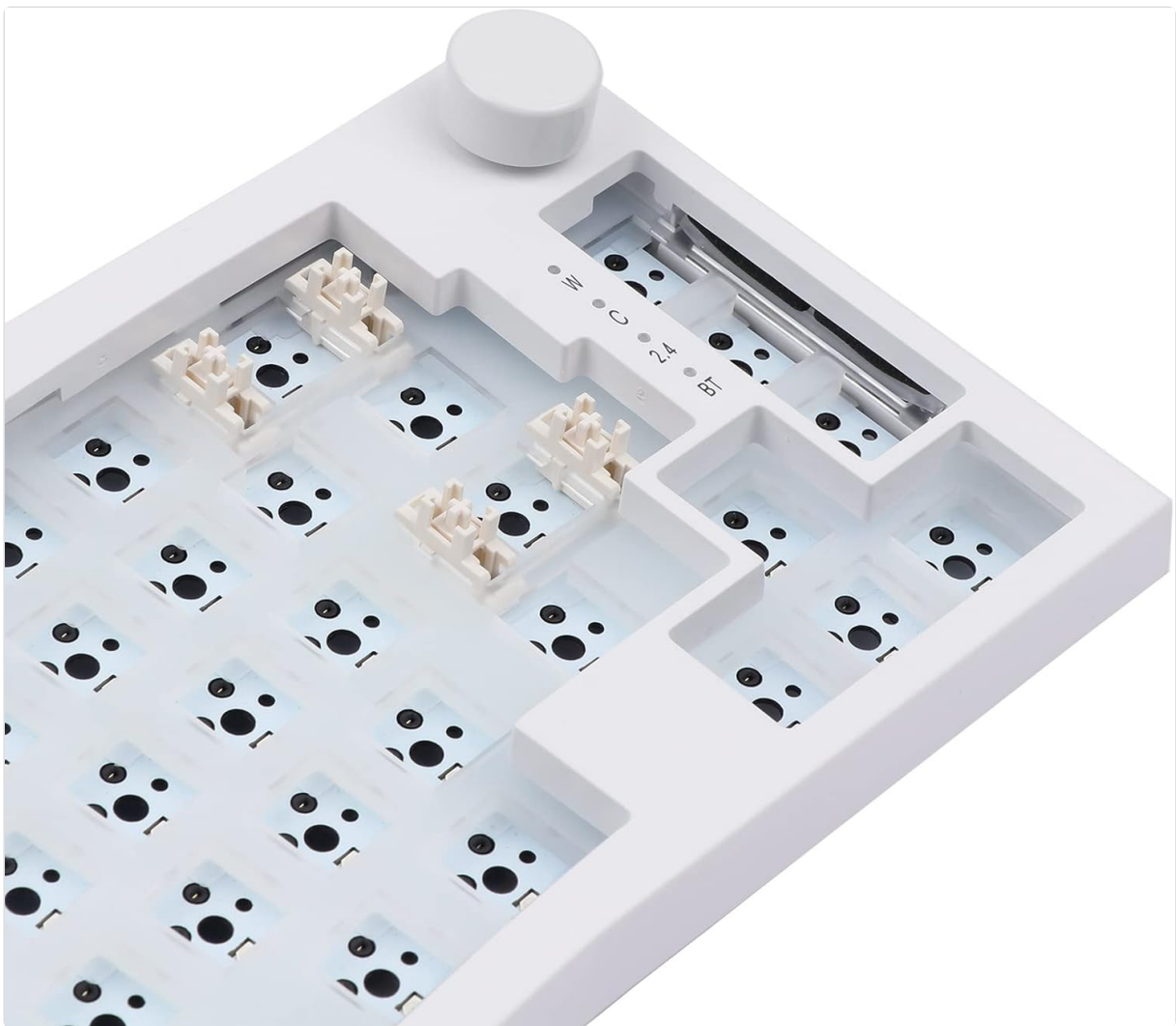
Image 3.2: A close-up view of the hot-swappable sockets on the Feker Alice 80 keyboard, ready for switch installation.
