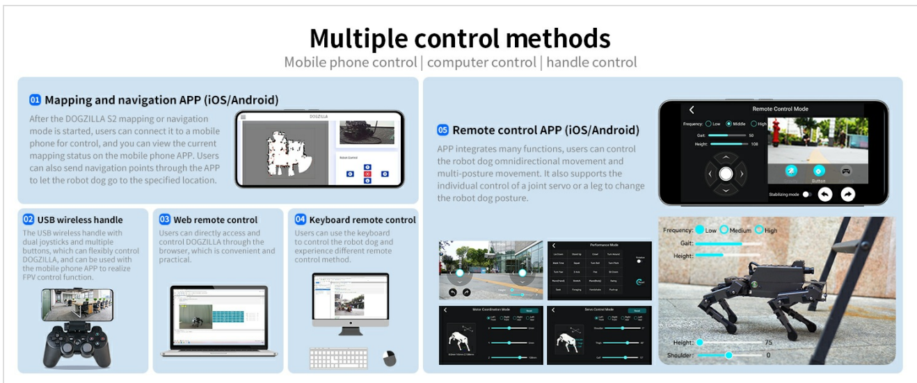
Figure 4.7: Different ways to control the DOGZILLA robot dog.
