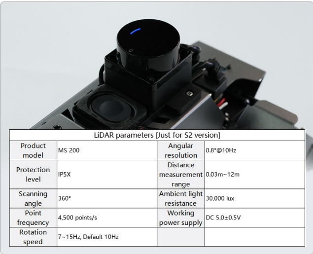
Figure 7.2: Close-up of the serial bus servo and a table of LIDAR parameters (LIDAR is for S2 version only).
