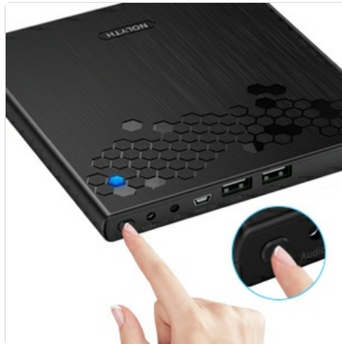
Image: Location and operation of the eject button.
