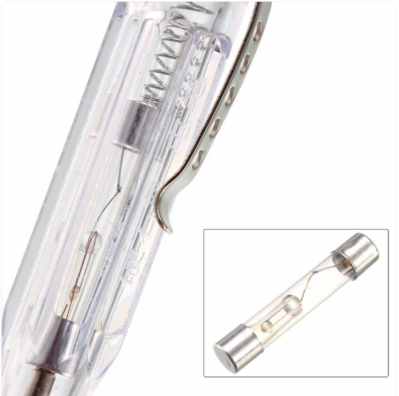
Figure 3.2: Internal Components (Neon Tube and Spring).
