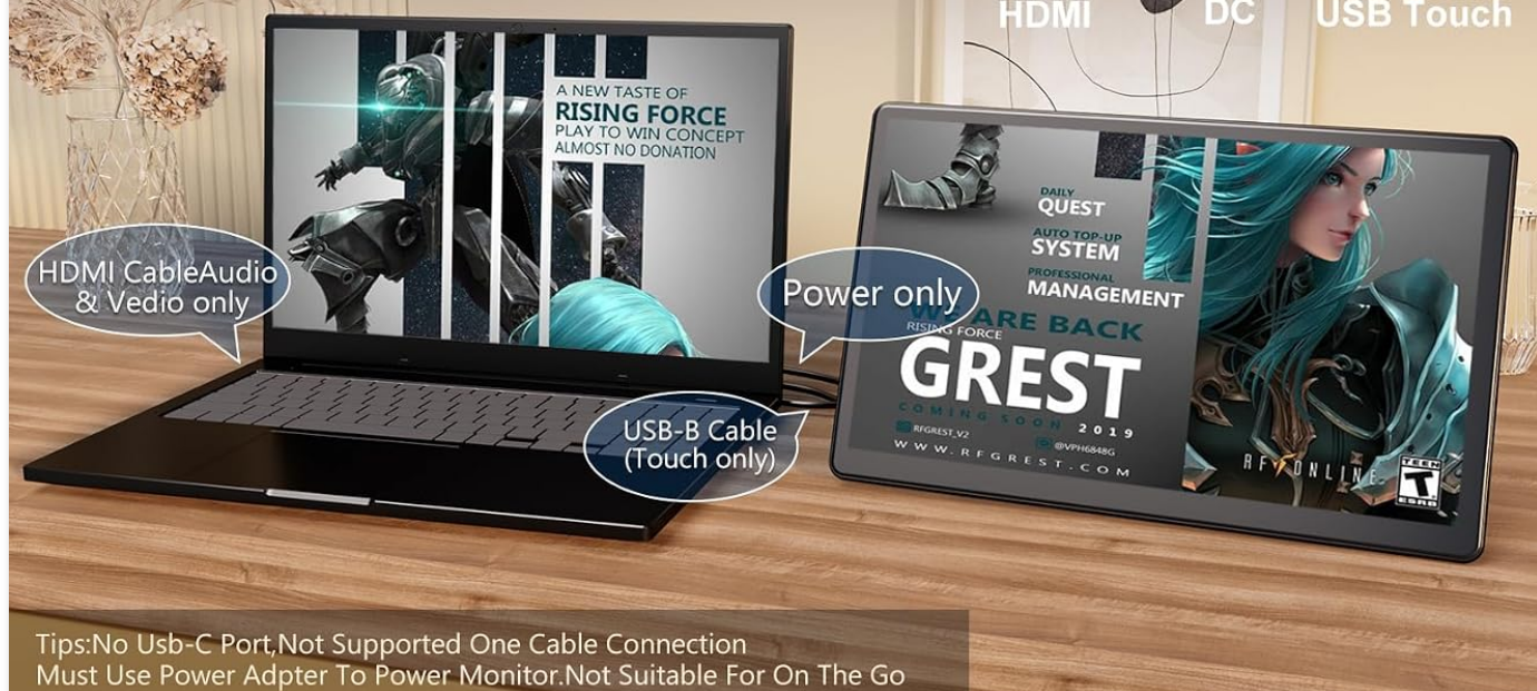
Image: Connection methods for non-touch and touch modes.
