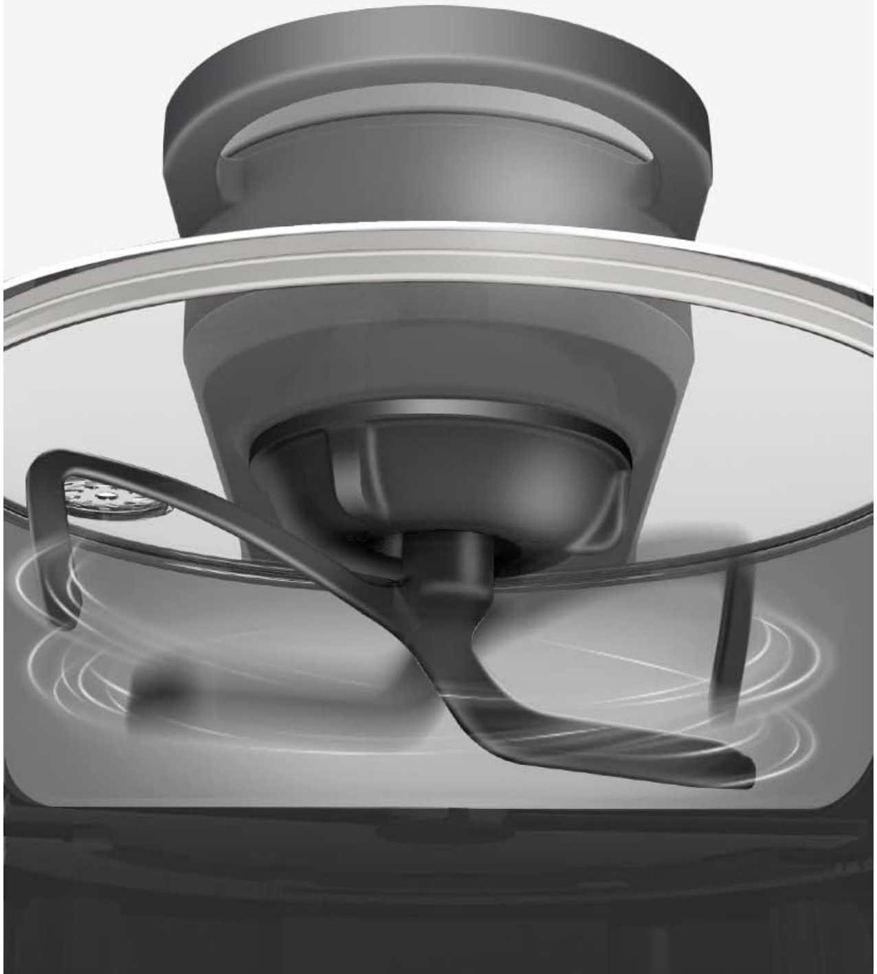
Figure 3.2: Close-up view of the internal double-wing stirring spatula. This component is responsible for automatically stirring ingredients during cooking, ensuring even distribution and preventing burning.
