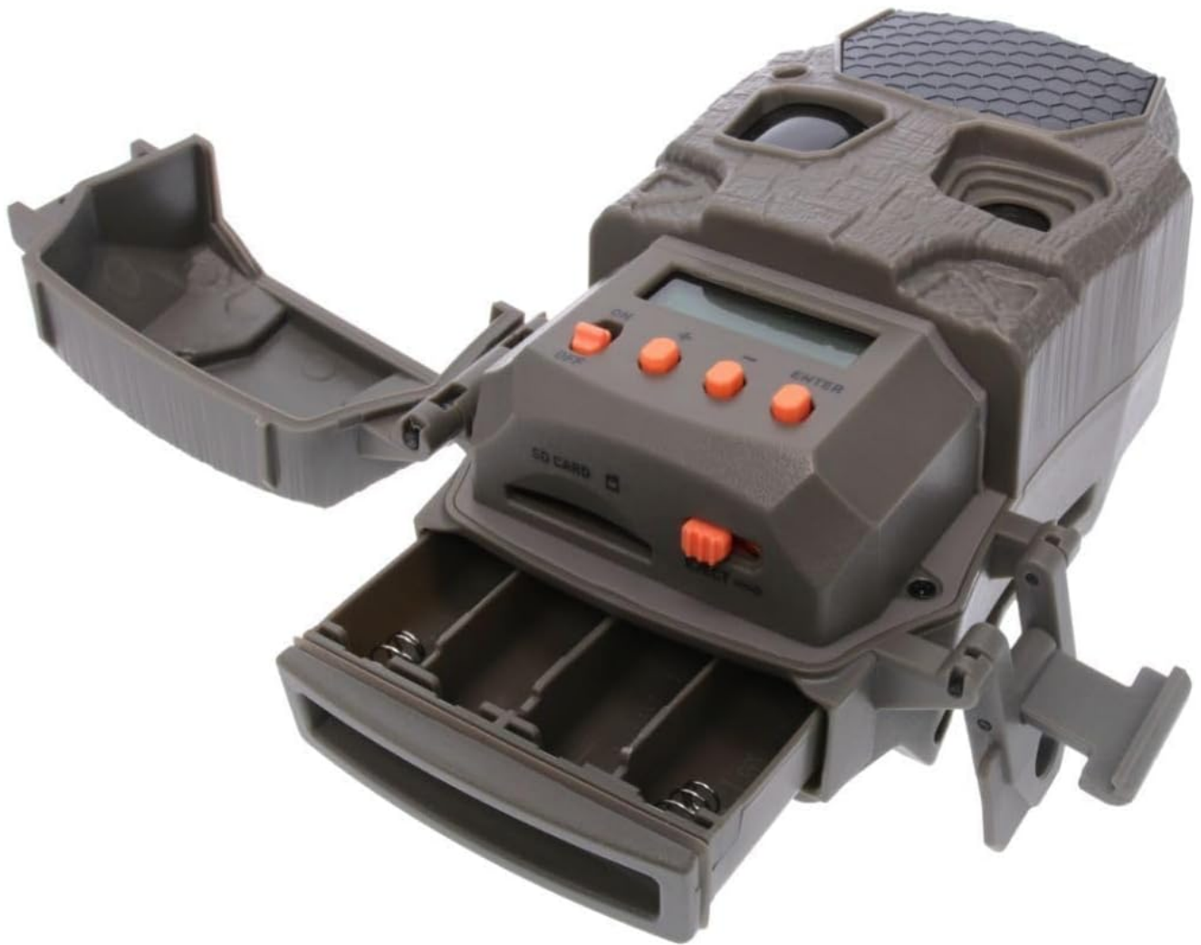
Image: Internal view of the Kicker 2.0 camera, highlighting the battery and SD card slots.
