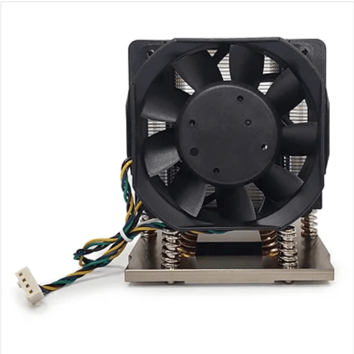
Figure 2: Front view of the Dynatron J12 heatsink, highlighting the fan and its connection cable.
