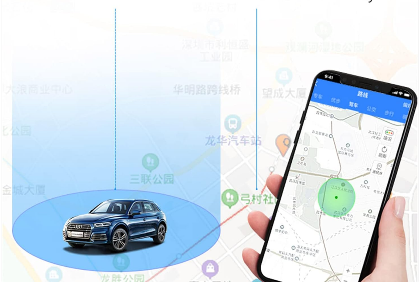
Image: A map interface on a smartphone showing a "safe area" and an "alarm range," with a car icon moving, illustrating how the geofence feature triggers alerts when the vehicle enters or leaves the set area.
