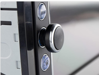
Figure 4: Detailed view of the physical controls on the left side of the unit, including the 'BND' button, rotary volume/selection knob, and the home button, providing tactile interaction points.
