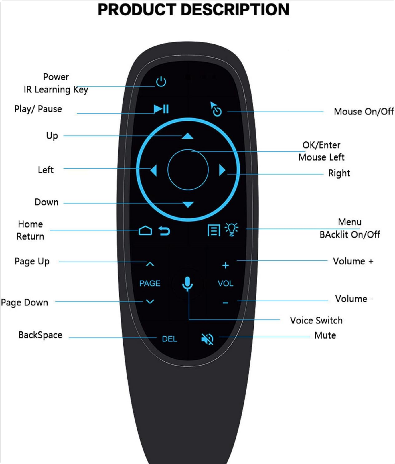
Image: A detailed diagram illustrating the function of each button on the Pomya G10S PRO BT remote control.
