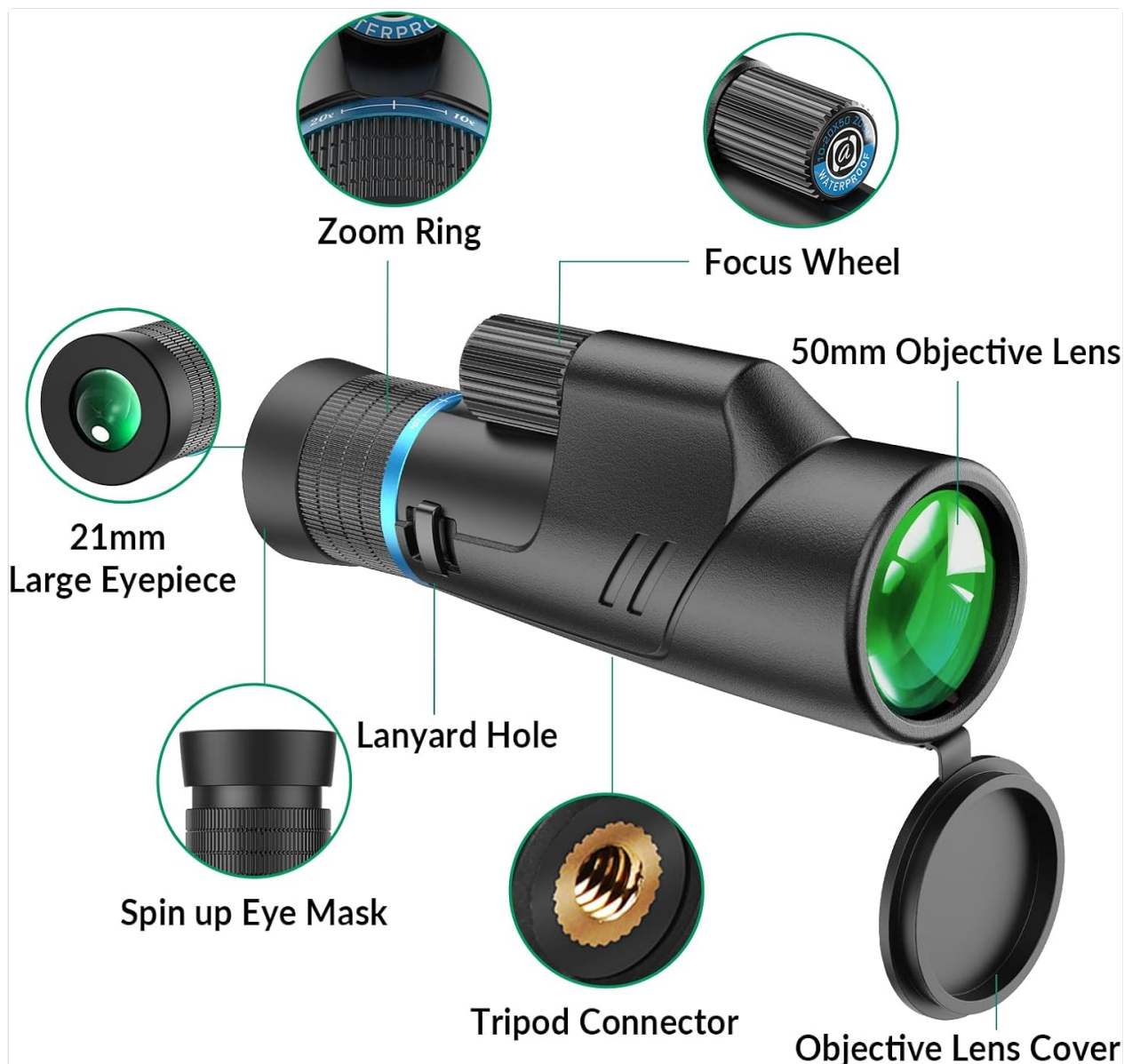
Image 2.1: Monocular Components
