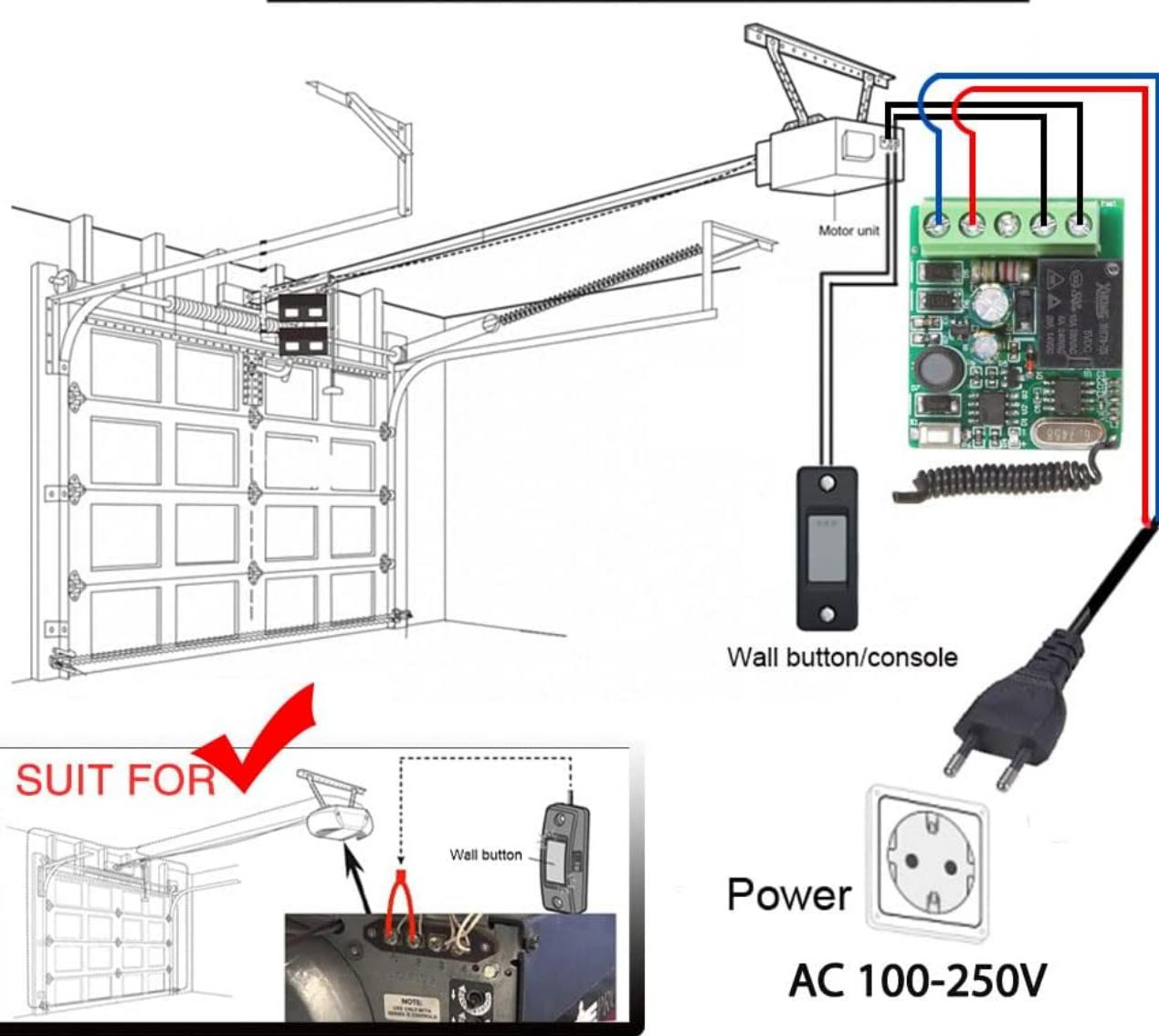
Image: Diagram showing the DieseRC receiver wired to a garage door opener motor unit and a wall button. The receiver's NO and COM terminals are connected in parallel to the wall button's terminals, allowing remote control of the garage door. The receiver is powered by AC 100-250V.
