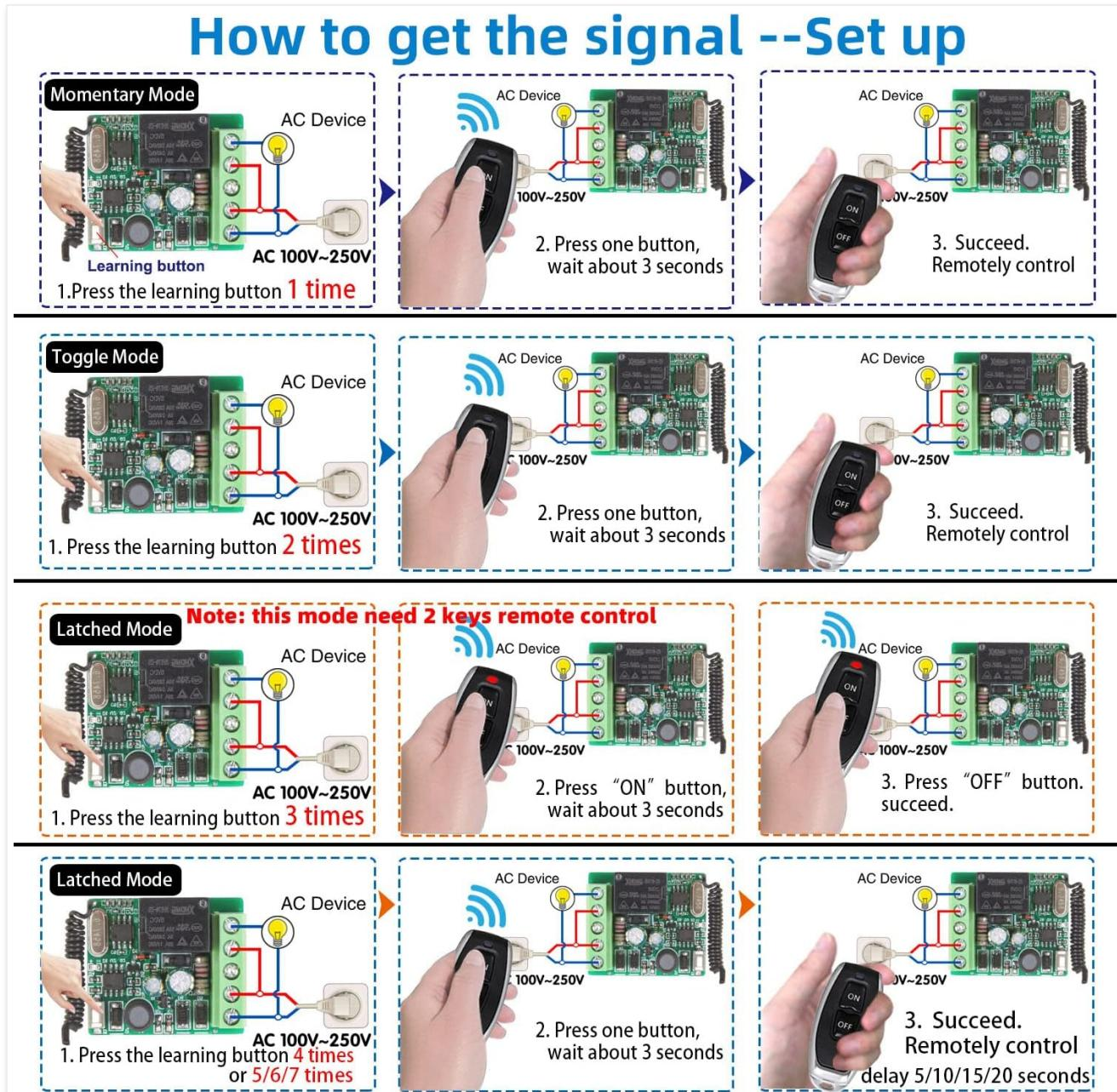
Image: Programming instructions for Momentary, Toggle, Latched, and Delay modes. Each section shows how many times to press the learning button on the receiver and which button(s) to press on the remote control to successfully set the mode.
