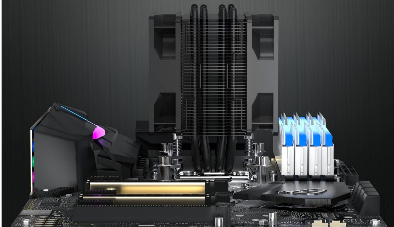
Image: The upHere A94K cooler installed, demonstrating excellent RAM clearance.
