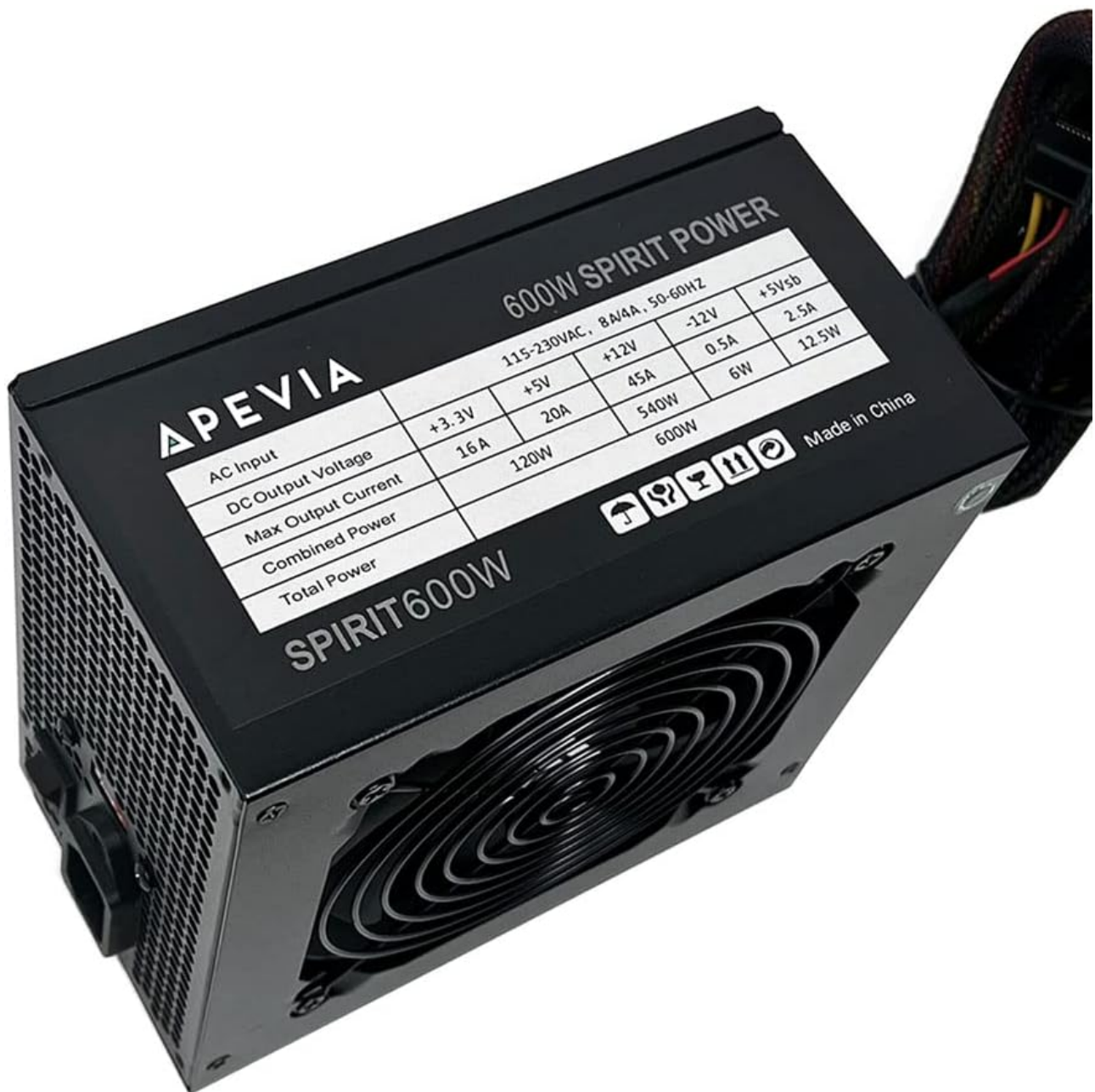
Figure 2.4: Detailed view of the specification label on the power supply, indicating input/output voltages and currents.
