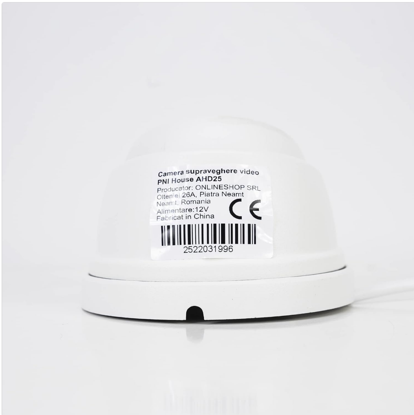
Image 9.1: Bottom view of the PNI House AHD25 camera, showing the product label with manufacturer details, voltage, and CE mark. The serial number is 2522031996 .
