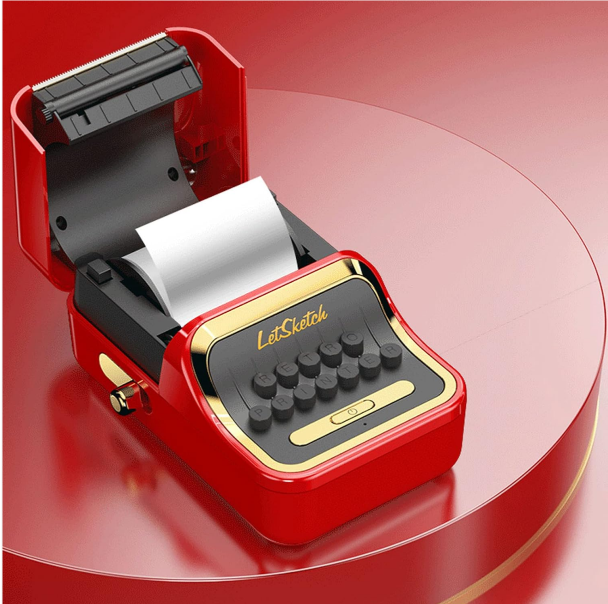
Figure 5.2: Loading labels into the printer compartment.
