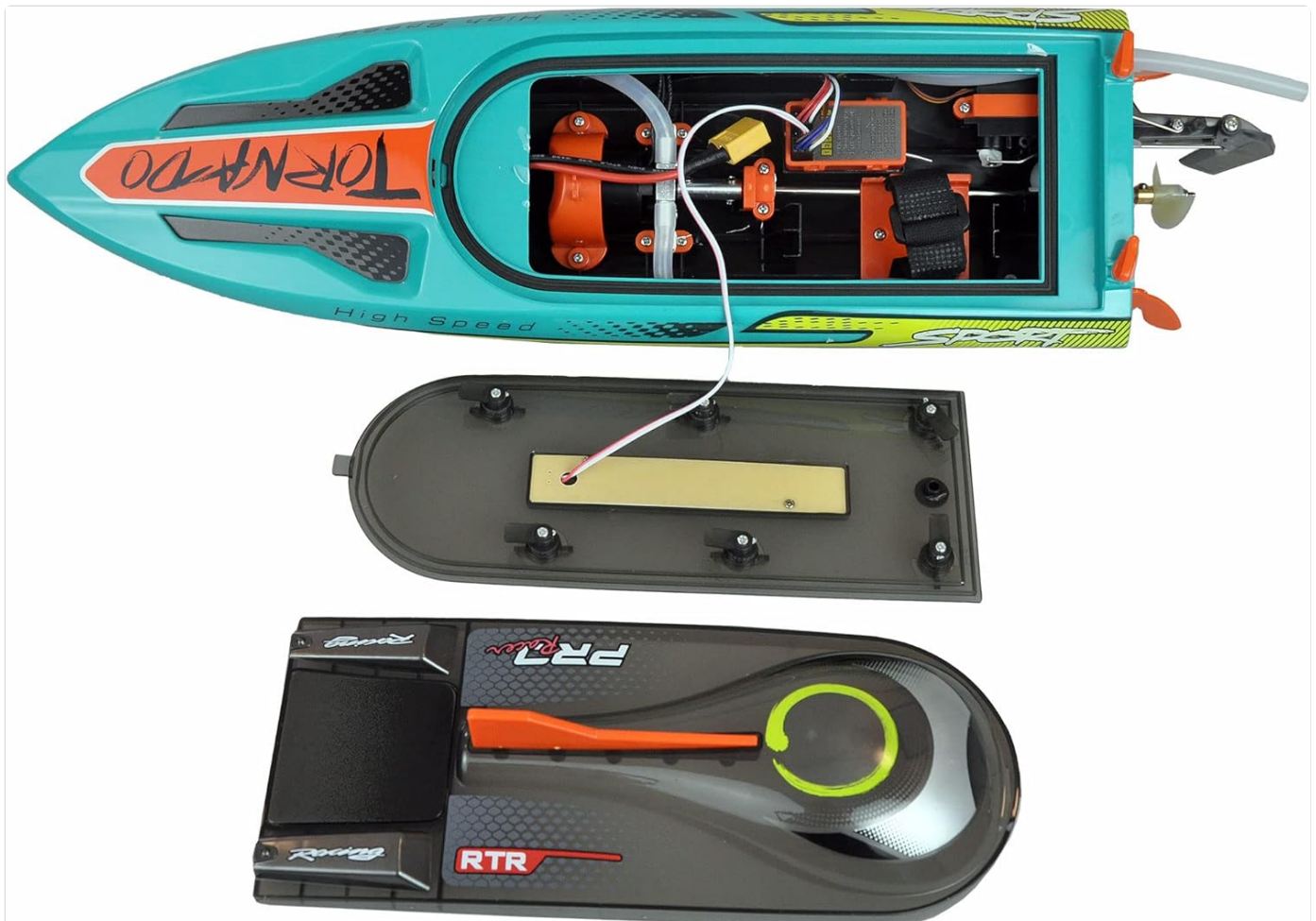
Image: Internal view of the boat's hull, showing the placement of the LiPo battery secured by straps and connected to the electronics.
