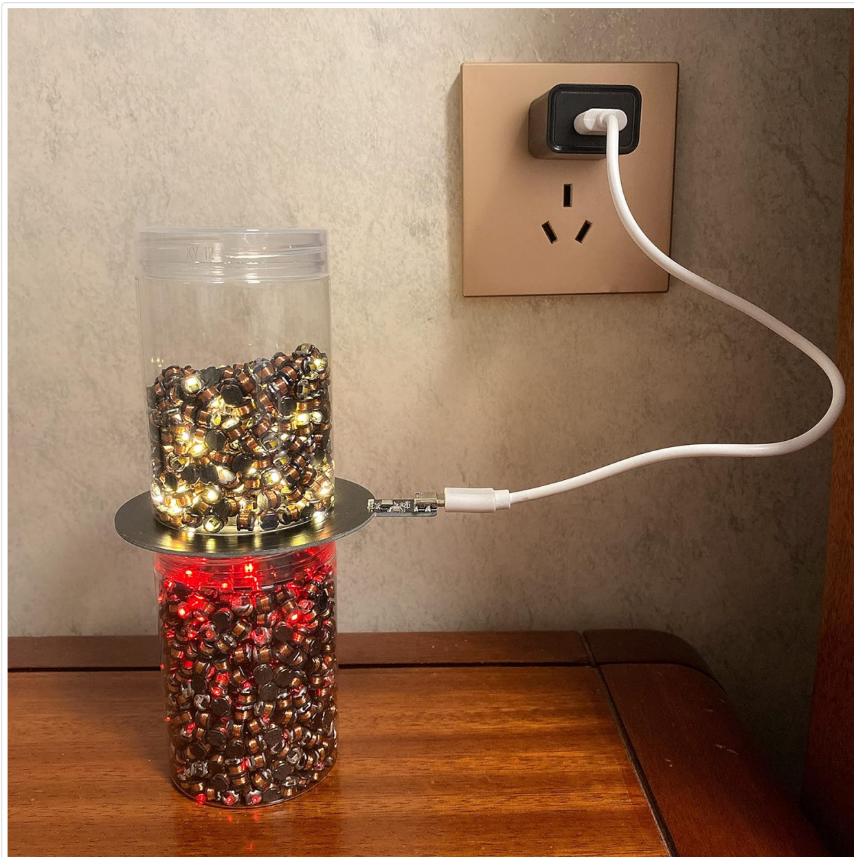
Image: The inductive PCB connected to a wall adapter, placed beneath a clear container filled with numerous small LEDs, which are all illuminated, demonstrating its use in a decorative setup.
