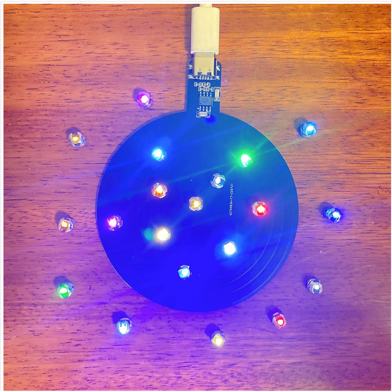
Image: The inductive PCB connected to a USB power source, with several small, colored LEDs glowing brightly around its surface, demonstrating wireless power transfer.
