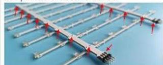
Figure 3.1: Step-by-step visual guide for soldering LEDs onto the PCB strips and assembling the cube layers.
