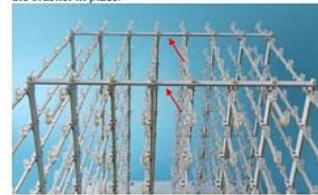
Figure 3.1: Step-by-step visual guide for soldering LEDs onto the PCB strips and assembling the cube layers.
