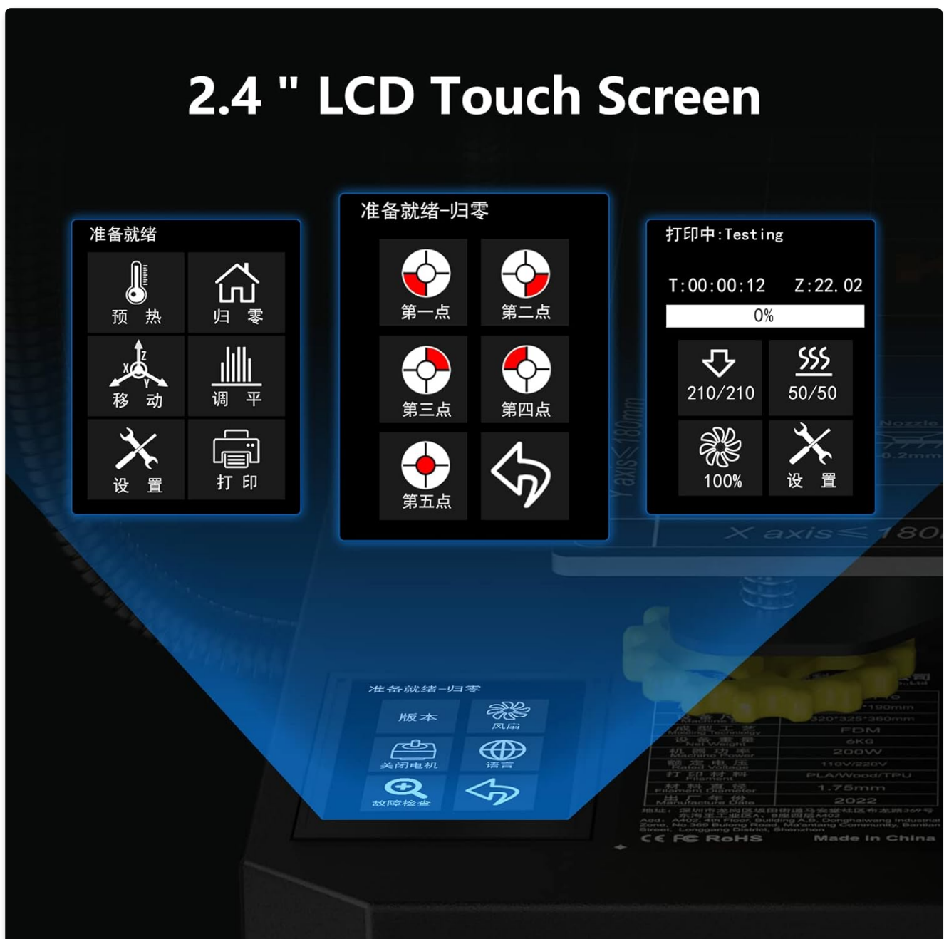
Figure 4: The 2.4-inch LCD touch screen displaying various control options including preheat, home, move, leveling, settings, and print functions.
