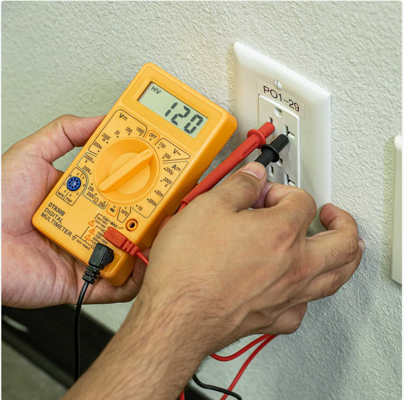
Image: A person using the multimeter to measure the voltage of a standard wall outlet. The multimeter's display shows a reading of "120", indicating 120 volts AC.
